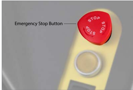
The Emergency Stop button.
